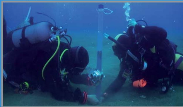
Sediment coring by PVC-Liner (LiSSa) for geotechnical analysis (SDC, 2011)
